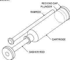
1. While holding the cartridge, grasp the dasher rod and extend it fully.
