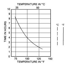
**Note**: Potted connectors or coatings of M-Coat J that exceed 3/8 in [10 mm] in thickness should be air dried for 30 minutes at room temperature prior to starting an elevated-temperature cure.
